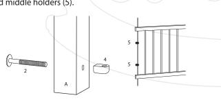
Insert the rods (8) into lower brackets (4) and fasten the screws (2). middle brackets (5) to crib bed (A, C)
