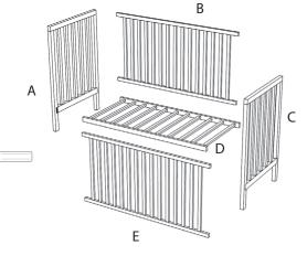
Using screws (1) and roller nuts (3), connect the front (A, C) and side parts (B)
