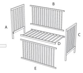
Using screws (1) and roller nuts (3), connect the front (A, C) and side parts (B)
