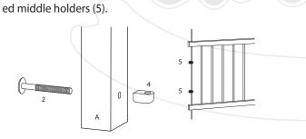
Insert the rods (8) into lower brackets (4) and fasten the screws (2). middle brackets (5) to crib bed (A, C)
