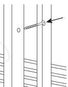
Attach the screws (2) to the lower brackets (4) in the lower part of the legsof both front walls and slide through into the pull-in side (E). Drilled holes metal rods (8), in the middle with thread-
