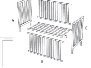
Using screws (1) and roller nuts (3), connect the front (A, C) and side parts (B)
